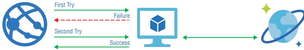
FIGURE 4.5 A retry cloud design pattern diagram
