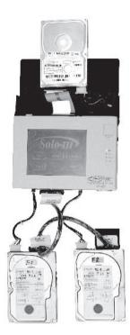
**Figure 2-4** The Image MASSter Solo-3 performs high-speed data acquisition.
