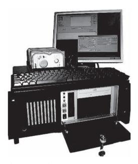
**Figure 2-11** The ImageMASSter 6007SAS performs high-speed data duplication over local or network connections.
