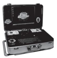
**Figure 2-6** The RoadMASSter-2 is used for data acquisition in the field.
