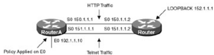
Figure 13-4: Application-level policy routing
